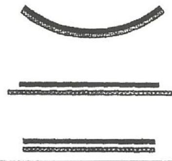
Fig. 5. The principle of the thermostat reveals how unequal expansion causes curvature. Strips of brass and iron of the same length (top) are heated separately (middle), and the brass expands more than the iron. If the strips are joined and heated, the brass strip curls around the iron one (bottom). Similarly, elongating plant cells curl around their less elongated neighbors. (Modified from P. S. Stevens, Patterns in Nature )
